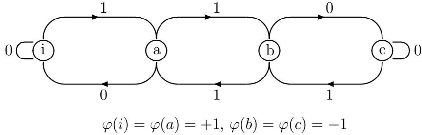
Figure 2: An automaton generating the Rudin-Shapiro sequence
